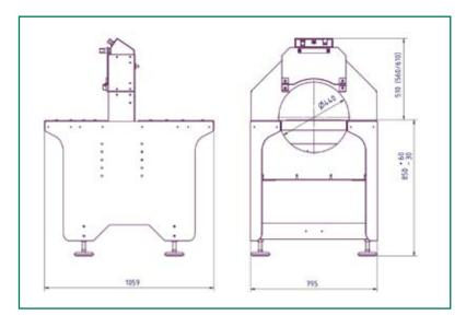
The wrapping head can be mounted at three heights.
